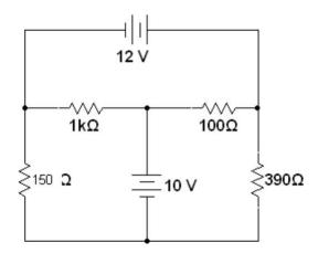
1. Conduct an experiment to determine the current through the  $100\Omega$  resistor for the given circuit using superposition theorem and compare with theoretical result
