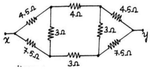
Solve for Vx&Vy using the super node concept for the circuit shown in Fig. (Apply)
